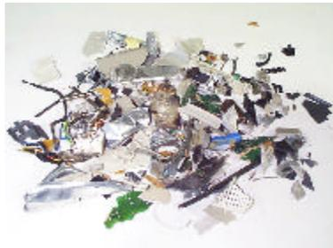
Shredded hard drives and other electronics processed by Cascade's new shredder.
