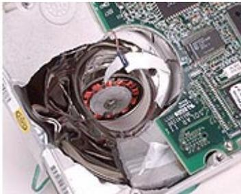
Hard drive run through Cascade's Mobile Crusher
