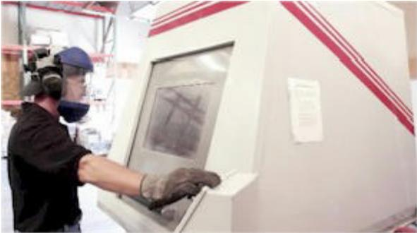
A Cascade employee operating the cathode ray tube cutter.
