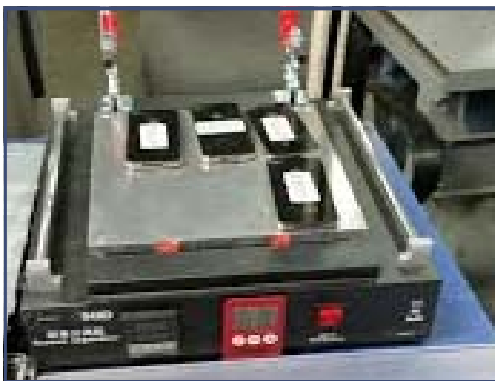
Hot plate used to aid in melting glue to access internal components in phones and tablets
