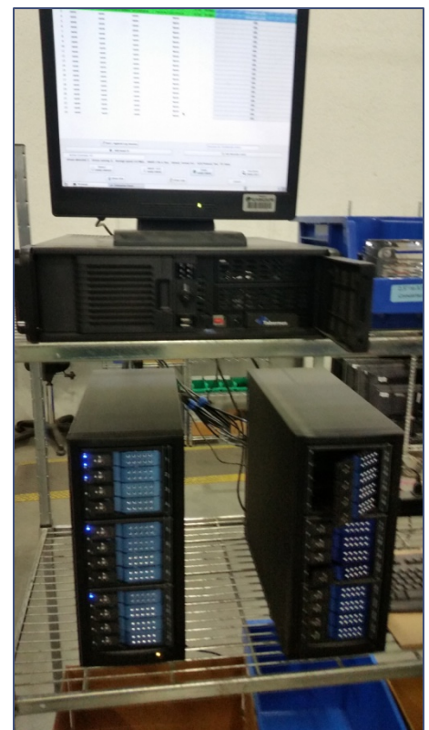
Drive array sanitization tool to allow for parallel wiping of servers drives, laptop drives, SSDs and more.
