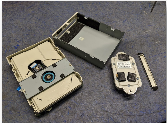
Tracking device (right) installed inside a disk drive sent to a Cascade downstream processor.
